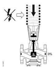
Figure 16. SQV91P40U Normally Closed Actuator.
