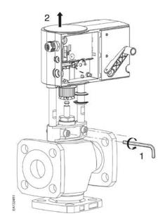
Figure 19. Removing the Actuator from the Valve.
