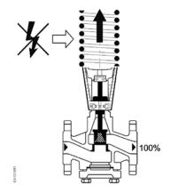
Figure 15. SQV91P30U Normally Open Actuator.
